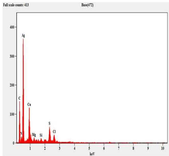
Figure 7: EDX spectra of synthesized silver nanoparticles
