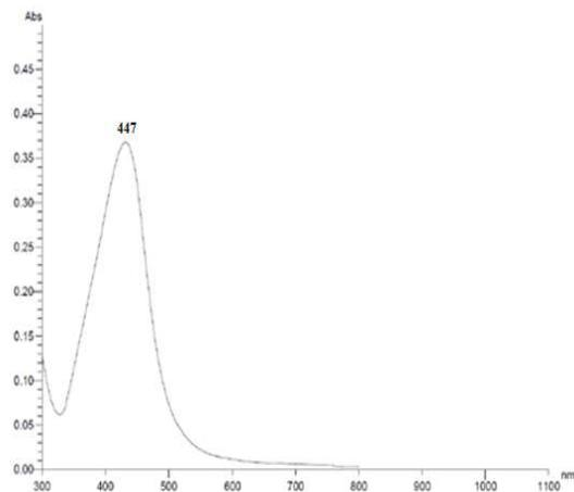
Figure 4: UV-Vis spectrum of produced Ag Nps
