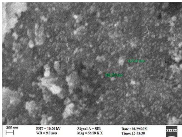
Figure 6: SEM image for synthesized silver nanoparticles
