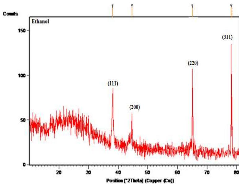
Figure 8: XRD patterns of silver nanoparticles synthesized using a sample
